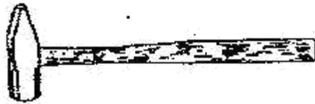
**Fig: Riveting Hammer**
