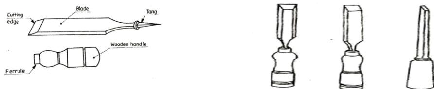
**Fig: Types of Chisels**
