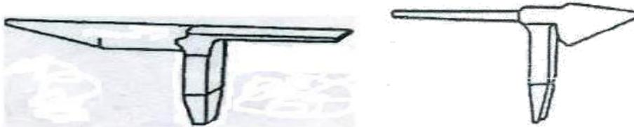
It is used for forming or seaming funnels. The below figure represents the blow horn stake:
